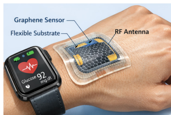
Figure 3. Example of a wearable graphene biosensor.
